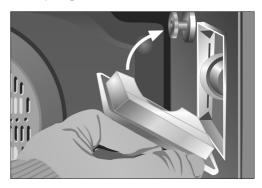
The replacement bulb must be resistant to temperatures up to 300  $^\circ\text{C}.$  You can order one from Technical Service.
